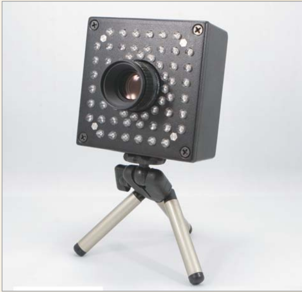
The eyebox2 is a portable, long-distance eye-tracking device that can be used for purposes such as determining the number of people who look at billboards. This could help identify the billboards' effectiveness. The eyebox2 emits infrared light and tracks reflections from viewers' eyes.
