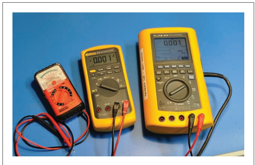
Figure 2. Evolution of a multimeter: an analog multimeter (left), a multimeter with LCD display (middle), and a multimeter with large screen display and analysis functions (right).
